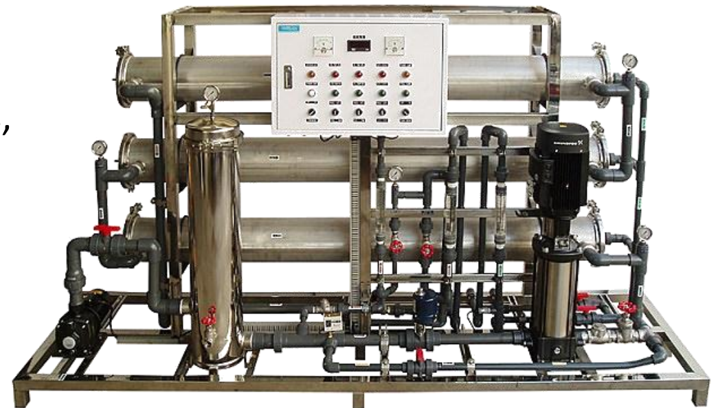
RO system takes small space due to its modularity.
